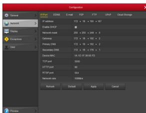
**NOTE :** modify the IP on the WAN interface for WiFi NVR with multiple network ports.
